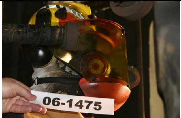
06-1475 A After Ignition of one strap on respirator which was unprotected by the faceshield
