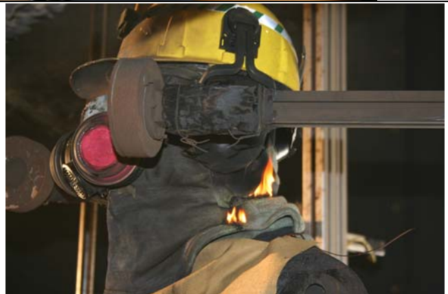
06-1475 A After Ignition of one strap on respirator which was unprotected by the faceshield
