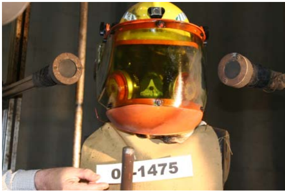
06-1475 A After Ignition of one strap on respirator which was unprotected by the faceshield
