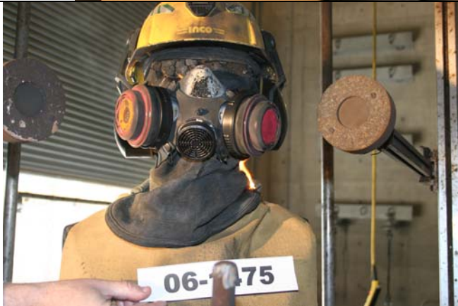
06-1475 A After Ignition of one strap on respirator which was unprotected by the faceshield
